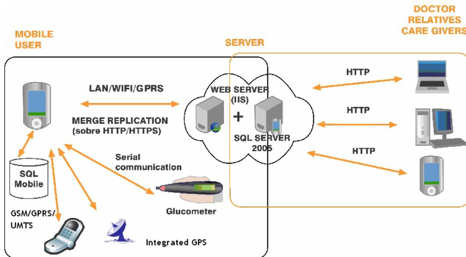
Fig. 3. Technical architecture of the entire system.
